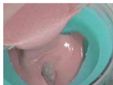
Wirovest refractory material being poured into the hydrocolloid mould made with Wirogel M.
