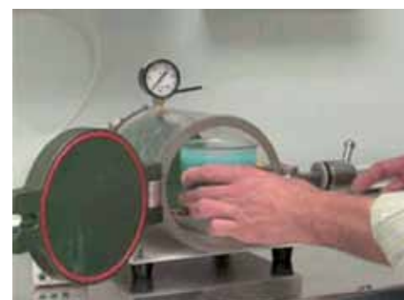
Place duplicated refractory model into the Wiropress SL pressure vessel, under 30psi of pressure.
